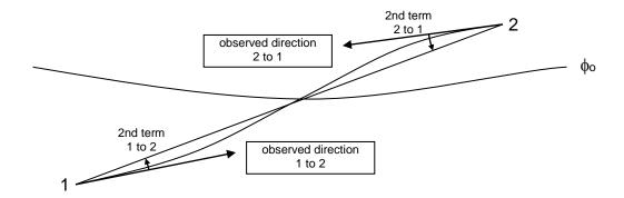
When the correction is applied to the observed geodetic azimuth, the proper azimuth value to use for calculating the coordinates of the forward point is obtained. Hence the equation for grid azimuth is...
