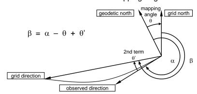
While the second term is shown with a "plus" sign, it must be remembered that it is added <u>algebraically</u>, and its actual sign depends upon the solution to the second term equation...
